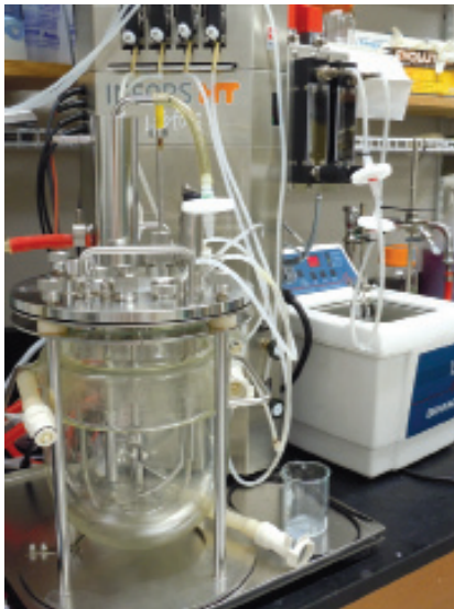
Bacterial fermenter used to cultivate electrogenic bacteria.
