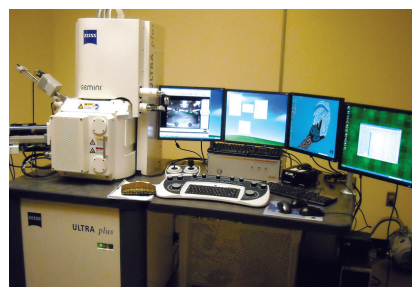
The Zeiss Ultra plus Field Emission Scanning Electron Microscope in the USC electron microscopy center.
