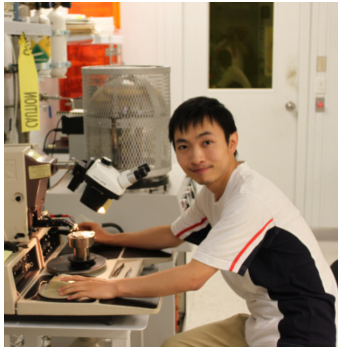
Ning (physics graduate) is using the wire bonding machine to bond gold wire into the sample.
